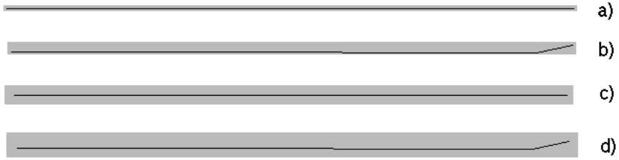
Fig. 2. Source raster lines and centerlines obtained with universal vectorization system A. Thickness of lines: a) 1 pixel, b) 2 pixels, c) 3 pixels, d) 4 pixels.
